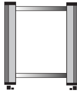
Pedestrian access units. Guarding by Safety Light Grids , body protection.
